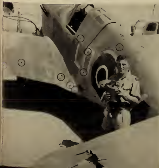
Even the Squadron Leader sometimes was caught unawares. Note the scars left by a 20 mm. cannon shell and machine gun bullets (holes circled).
